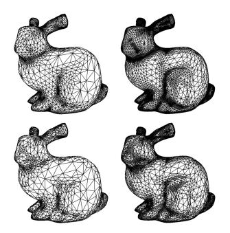
Figure 12: Adaptive refinement based on red-green triangulation with Loop subdivision (top row) and based on the  $\sqrt{3}$ -refinement (bottom row). While the same stopping criterion is used (left and right respectively), the Loop meshes have 10072 and 28654 triangles while the  $\sqrt{3}$ -meshes only have 7174 and 20772 triangles.
