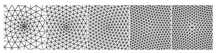
Figure 17: The local regularity of the subdivision surface at extraordinary vertices requires the injectivity of the characteristic map. We show the isoparameter lines for these maps in the vicinity of irregular vertices with valence n = 3, 4, 5, 7, and 8 (form left to right).
