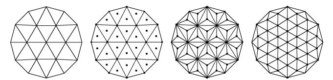
Figure 2: The  $\sqrt{3}$ -subdivision scheme is based on a split operation which first inserts a new vertex for every face of the given mesh. Flipping the original edges then yields the final result which is a 30 degree rotated regular mesh. Applying the  $\sqrt{3}$ -subdivision scheme twice leads to a 1-to-9 refinement of the original mesh. As this corresponds to a tri-adic split (two new vertices are introduced for every original edge) we call our scheme  $\sqrt{3}$ -subdivision.
