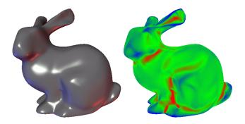
Figure 10: A decimated Stanford bunny was used as a subdivision control mesh  $\mathcal{M}_0$ . We applied the  $\sqrt{3}$ -subdivision scheme 4 times (left). The right image shows the mean curvature distribution.
