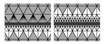
Figure 6: The gap fixing by triangle fans tends to produce degenerate triangles if the refinement is not balanced (left). Balancing the refinement, however, causes a larger region of the mesh to be affected by local refinement (right).
