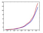
Figure 11: This plot shows the triangle count  $(Y : in K \triangle)$  vs. approximation error  $(X : in - \log(\varepsilon))$ . The red curve is the complexity of the Loop-meshes, the blue curve the complexity of the  $\sqrt{3}$ -meshes. The ratio lies between 5% and 25%.
