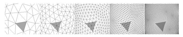
Figure 3: The  $\sqrt{3}$ -subdivision generates semi-regular meshes since all new vertices have valence six. After an even number 2k of refinement steps, each original triangle is replaced by a regular patch with 9<sup>k</sup> triangles.
