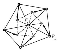
Figure 4: *The application of the subdivision matrix S causes a rotation around* **p** *since the neighboring vertices are replaced by the centers of the adjacent triangles.*
