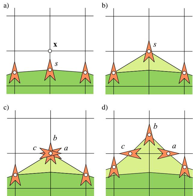
**Fig. 9** Splitting snaxels: a) Original r-snake. b) Snaxel  $s$  has run into gridpoint  $x$  from the south. c) Snaxel  $s$  is split into three new snaxels  $a, b, c$  that run to the east, north and west respectively. d) Some timesteps later.
