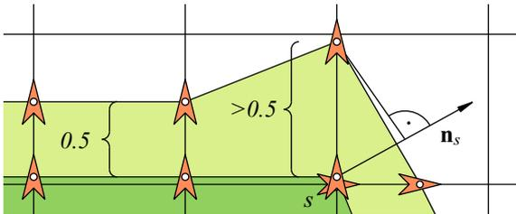
**Fig. 6** A contour evolving with unit speed  $v \equiv 0.5$  may nevertheless develop cusps because of the arbitrary approximation of the normal  $\mathbf{n}_s$  of the snaxel  $s$ .
