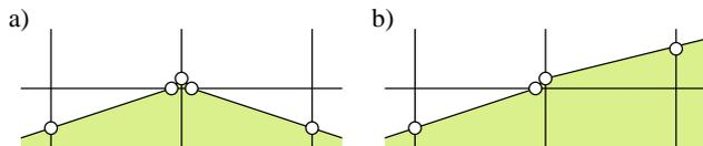
**Fig. 11** Multiple vertices: Triple (a) and double (b) vertices may appear after a snaxel split. Although these vertices share the same spatial position, they are conceptually distinct, as they are supported by different grid segments. Due to the parameter independent evolution rule this degenerate snake parameterization does not affect the numerical robustness of the algorithm.
