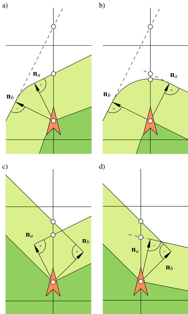
**Fig. 8** Snaxel speeds are computed by applying Huygen's principle on continuous contours: The original contour (dark) is locally propagated with constant speed. The intersection points of the resulting continuous offset contour (light) with the grid are then used to determine the new snaxel positions of the original contour.
