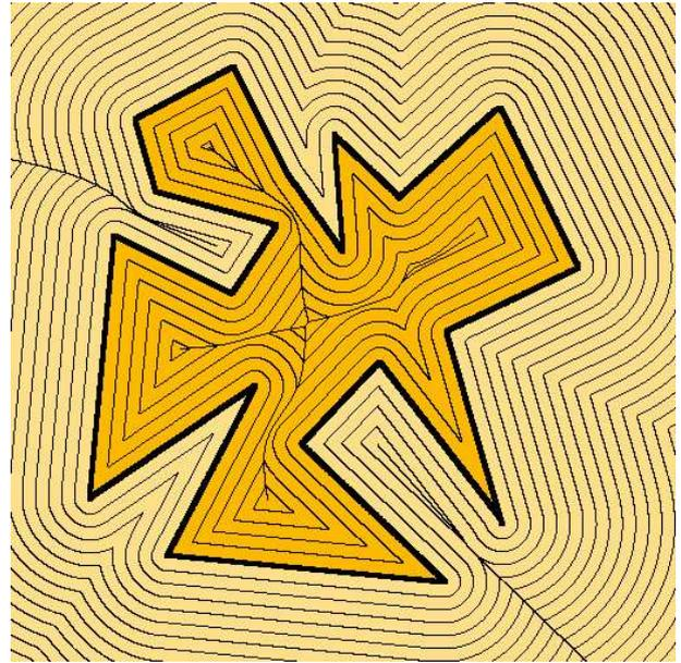
**Fig. 15** Contour evolution: The image above shows the evolution of two contours that were initialized as the inner and outer boundary of the polygon. Both contours propagate with unit speed  $v \equiv 1$  and are shown at equidistant time intervals. The resolution of the underlying grid is  $512 \times 512$ .
