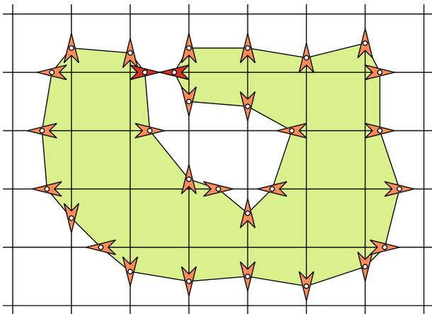
**Fig. 4** A typical r-snake: Note that the two darkened snaxels share the same supporting segment. Such a sub-pixel configuration could not be modeled with snakes in level set formulations [11].
