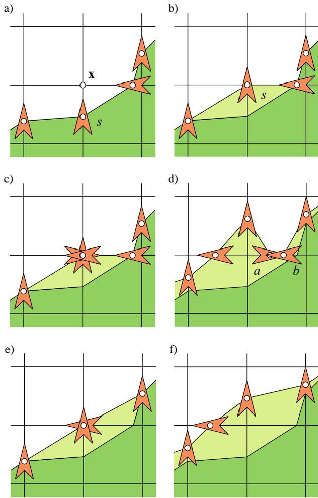
**Fig. 10** Cleaning conquest: a) Original r-snake. b) Snaxel  $s$  has run into gridpoint  $x$ . c) Snaxel  $s$  is split into three new snaxels. d) Without a cleaning conquest both snaxel  $a$  and snaxel  $b$  would violate condition 3. e) Snaxels  $a$  and  $b$  are removed by the cleaning conquest. f) Some timesteps later.
