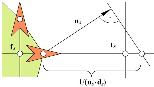
**Fig. 5** Projecting the snaxel speed: As snaxels can only move along their supporting segments, the normal speed has to be projected onto the segment.
