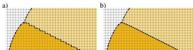
**Fig. 17** Ripples: When two r-snakes clash together, there may appear ripples in the order of one pixel’s magnitude (a). These ripples can be removed in a post-processing step by smoothing the r-snake (b).
