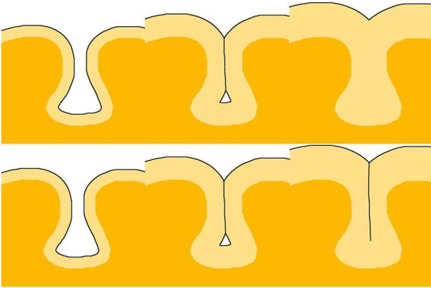
**Fig. 14** Depending on whether frozen snaxels are removed by the cleaning conquest, recesses will disappear as soon as they completely touch each other (top) or are conserved (bottom).
