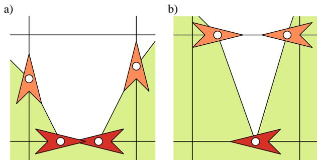
**Fig. 3** Forbidden snaxel configurations: The configurations shown above are forbidden, as the darkened snaxels point from the interior to the interior of the contours.
