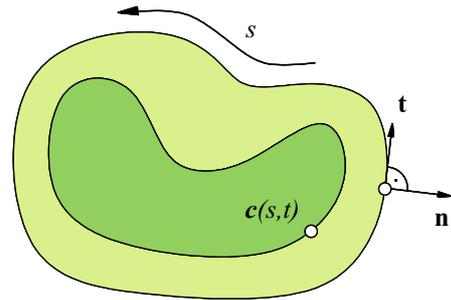
**Fig. 1** Evolving contours: A contour  $\mathbf{c}(s, t)$  is parameterized by arc length  $s$  and time  $t$ . The movement of each contour point  $\mathbf{c}(s, t)$  can be decomposed into tangential and normal components. Whilst the tangential component affects the parameterization of the contour, only the normal component modifies the contour’s shape.
