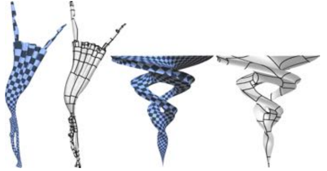
Fig. 17. Models on which the method of [Myles et al. 2014] is not able to respect the input signature. Shown are seamless similarity parametrizations and exemplary derived coarse T-meshes (not optimized for alignment or refined for any particular purpose) constructed by our method, with exactly the prescribed extraordinary vertices.
