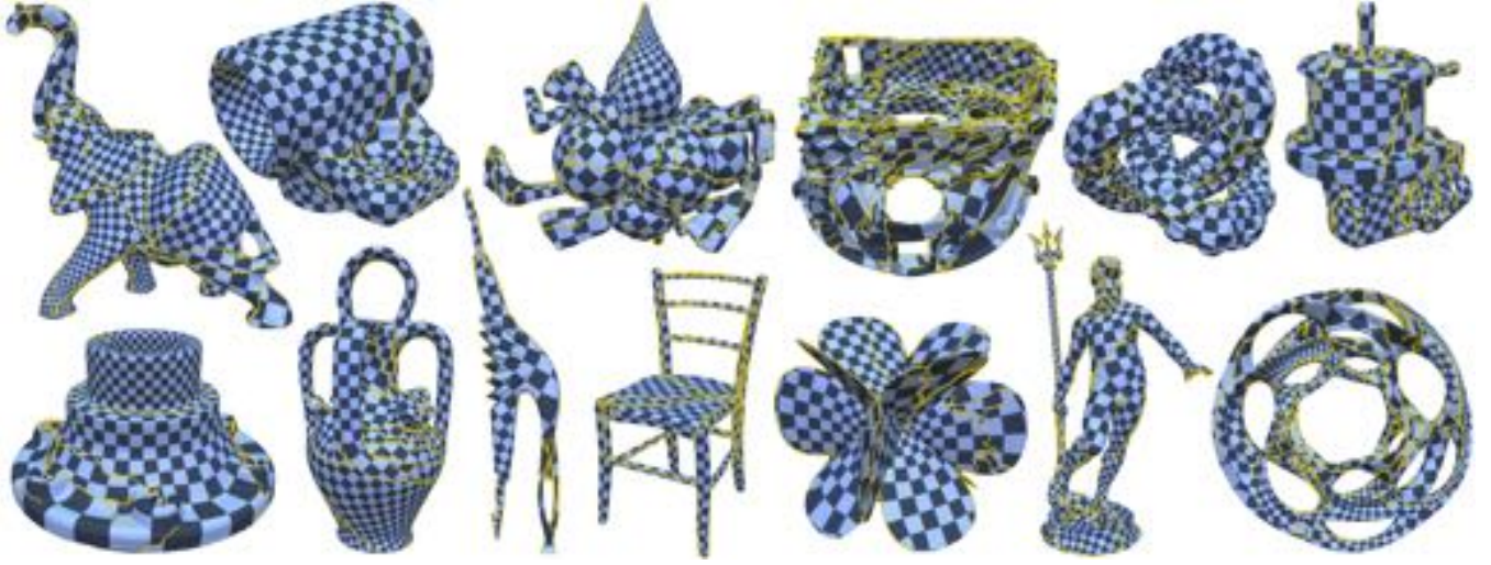
Fig. 16. Examples of conformal seamless similarity parametrizations, visualized with a checkerboard texture, as computed by our method. The cuts (across which the parameters are related by seamless similarity transformations) are highlighted in yellow.
