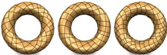
Fig. 5. T-spline surfaces (with superimposed images of the underlying control meshes) without extraordinary vertices. They differ in their holonomy signature (intuitively: the rotation of the control mesh ‘edge flow’ around the object). Only the left-most instance can be handled by seamless maps and classical T-splines with edge knots. Our variant with halfedge knots supports all three signatures (as well as any other).
