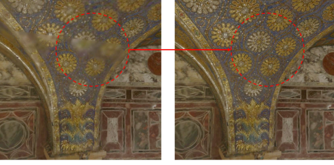
Fig. 2. Example of LOD popping . The marked region on the left appears to be blurred because no high-detail mipmap is resident for that page. In the next frame (on the right), the mipmap is available and the blurred region suddenly disappears. This effect can be very noticeable for users.
