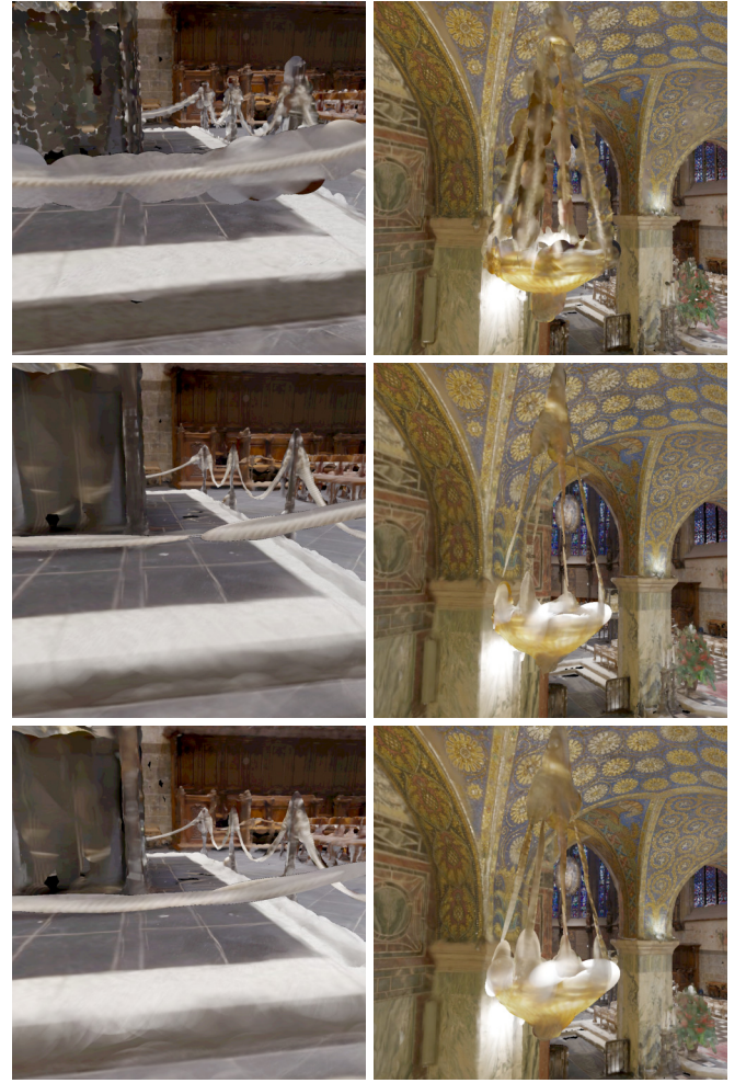
Fig. 6. Comparison of splatting primitives: Uniform-sized disc splats in the first row illustrate the difficulty to find an adequate global splat size. 2D ellipses in the second row improve the result, but fail to capture object contours from all viewing angles. Finally, our 3D ellipsoid splats in the third row achieve a plausible object contour from all viewing angles.
