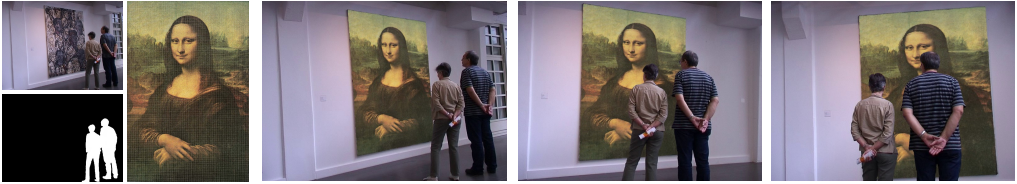
Figure 1: Our video editing system is built upon a pure 2D interface and is based on standard homography matching. Each tracked region can be easily modified in one frame and this new information, e.g. here a painting, can automatically be propagated through the whole video, thus creating the desired 3D effect.
