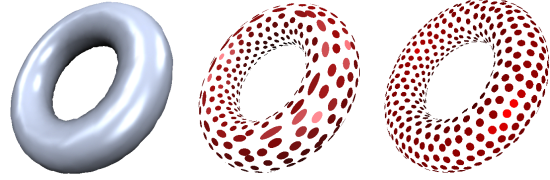
Figure 4: A torus approximated with error tolerance 0.2% by 510 elliptical splats (left and center) and by 734 circular splats (right).
