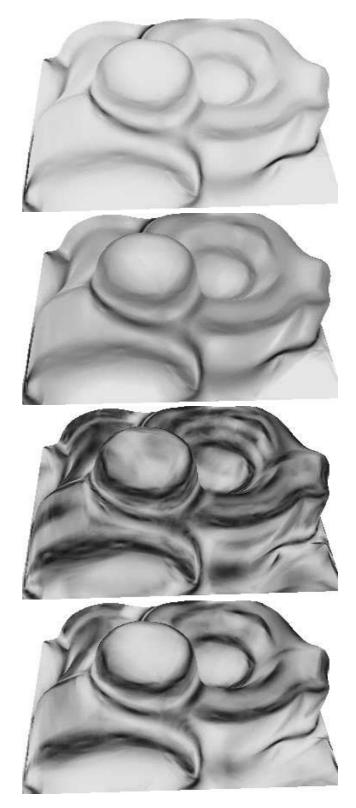
Figure 5: Median filtered maximal curvature on a technical model. From upper left to lower right: global color table with  $\gamma = 1$ ,  $\gamma = \frac{1}{2}$ ; local color table with  $\gamma = 1$  and 3-neighborhood resp. 6-neighborhood.
