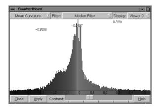
Figure 6: Snapshot of a histogram window. Median filtered mean curvature is selected, contrast is set to about 0.3, the interesting interval has been refined to about [-0.3, 0.3], and the zero/green level has slightly been moved to about -0.02.
