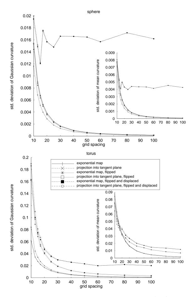
Figure 2: Approximization errors. First row: Sphere. Gaussian (large) and mean curvature (small); second row: Torus. Gaussian (large) and mean curvature (small)
