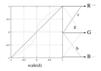
Figure 3: Color coding. d is mapped to [-1, 1] by **scale**, resolution near 0 may be enhanced by using  $\gamma < 1$  (left), the transformed value is then coded as (r, g, b) (right).
