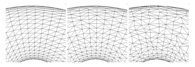
Figure 1: Triangulated torus with  $50 \times 50$  parameter points. From left: regular mesh, randomly flipped edges, flipped edges and random displacement of parameter points
