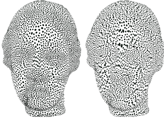
Figure 4: Igea model (134K points) coarsified to same number of 13K splats using L^2 error metric (left) and L^{2,1} metric (right) with respective run time 52 sec. and 31 sec. and relative Hausdorff distance error 0.017% and 0.022%.
