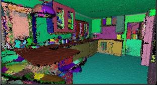
Figure 10 Segmentation results on a noisy indoor point cloud captured by a hand-held laser scanner Zeb-Revo
